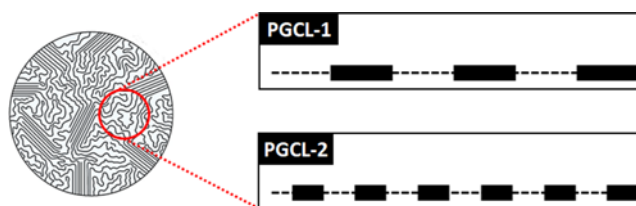
Figure 4. Schematic model of PGCL block copolymer with different sequence lengths at the same glycolide content.
