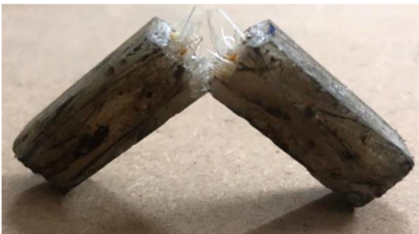
Figure 13. Impact fractured composite specimen.
