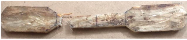
Figure 8. Tensile fractured specimen.
