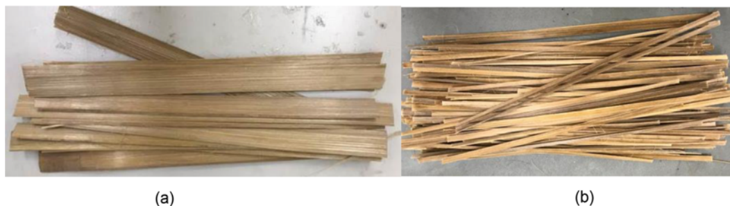
Figure 1. (a) Bamboo slices (b) bamboo strips in 0.7 \times 4 \times 160 \text{ mm}^3 .
