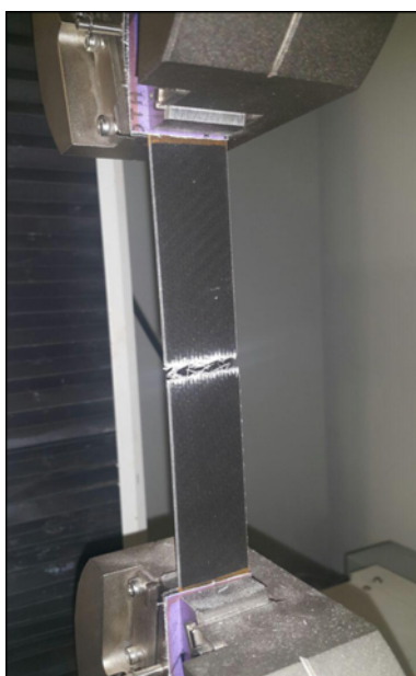
Figure 2. Nanocomposite specimen broken during the tensile test.
