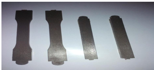
Figure 3. Composite samples to test tensile and flexural strength.
