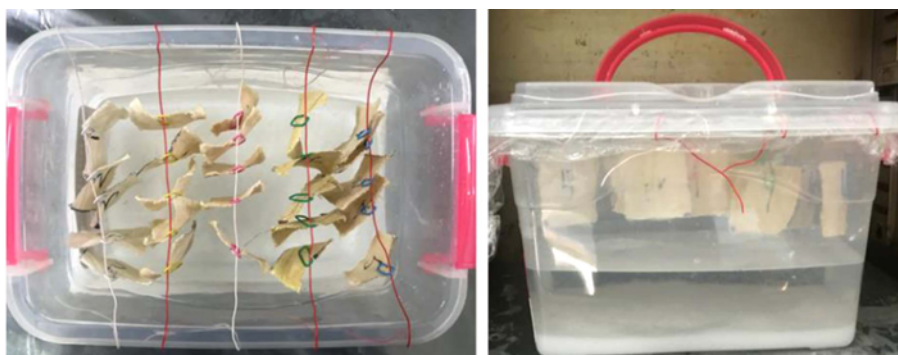
Figure 3. Flax fabric suspended in a box with the predetermined hydrothermal condition.
