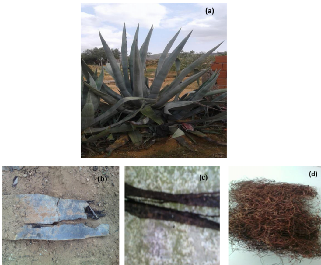
Figure 1. (a) Agave americana L plant, (b) leaves of Agave americana L before burial, (c) leaves after burial (decomposition of a natural matrix), and (d) the obtained fibers.
