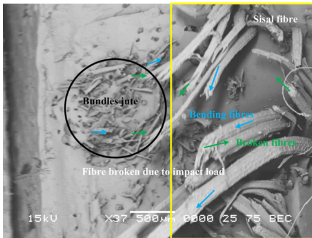
Figure 11. Fracture surface of the flexural test in hybrid composites (HCE02).
