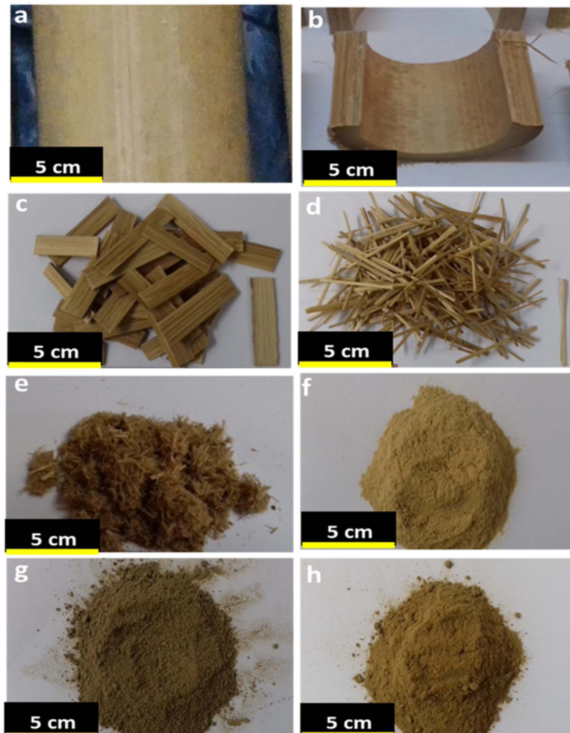
Figure 1. Conditions of (a) bamboo, (b) raw-cut, (c) chipped, (d) fine chipped, (e) ground, (f) milled - untreated BF, (g) SE BF, and (h) SE-alkali treatment BF.
