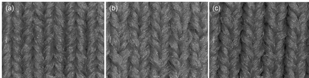
Figure 3. Changes in the structure of (a) the unwashed jersey fabric 1 (RS) upon (b) biaxial SL5 and (c) SR110 (technical face, magnification 3x).
