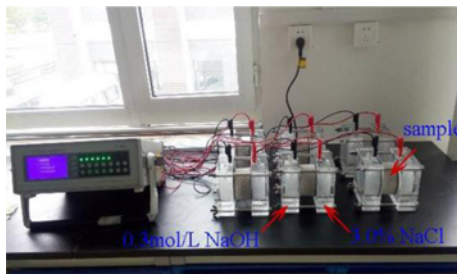
Figure 3. Rapid chloride penetration test.
