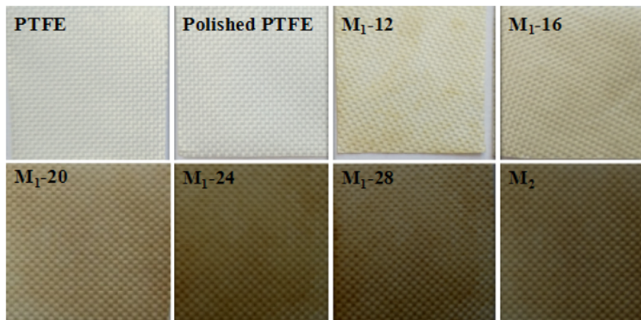
Figure 2. Surface colour of PTFE-fiberglass composite film under different treatment methods and processing time.
