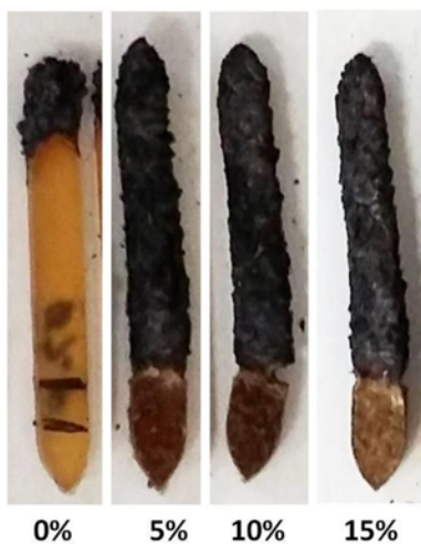
Figure 5. Behavior evaluation by flame test of matrix and biocomposites.
