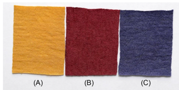
Figure 12. The coloration sample of the obtained cationic reactive dye 1 (A), 2 (B), 3 (C) on wool/acrylic blend fabrics.
