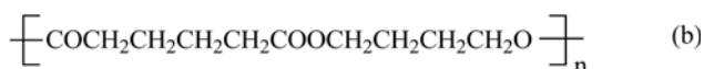
Scheme 1. The structures of (a) hard segments and (b) soft segments for TPU.
