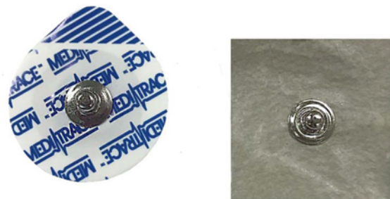
Figure 2. ECG electrodes: Conventional Ag/AgCl electrode (left) and AgNW/PU nanoweb electrode (right).
