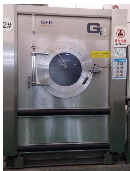
Figure 1. G2, an industrial plasma machine for color fading (photo obtained with permission).
