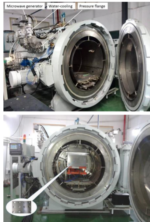
Figure 6. High-pressure microwave curing equipment.
