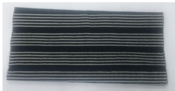
Figure 3. Knitting design and knitting electrode for the electrode configuration.
