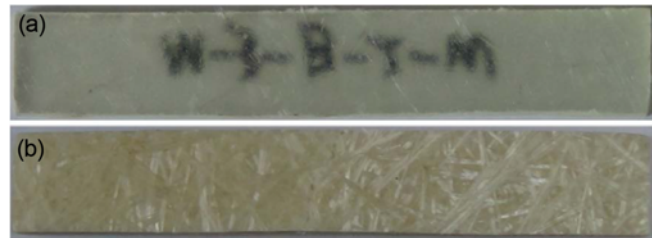
Figure 17. Photos showing the surfaces for hybrid composites 3-W subjected to different water immersion duration; (a) 0 day and (b) 90 days.
