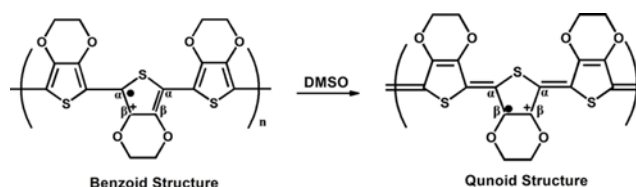
Scheme 1. Transmission of PEDOT chain from benzoid to quinoid structure.
