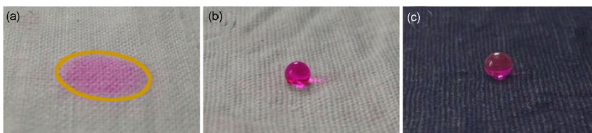
Figure 4. Photographs of water droplet on pristine cotton (a), (b) cotton with Nafion-MWCNTs, cotton with Nafion only (c).
