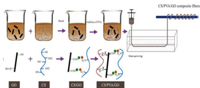
Figure 1. The prepared process of water-soluble CS/PVA/GO solution and continuous CS/PVA/GO composite fibers by wet-spinning assembly.
