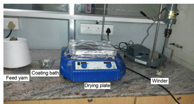
Figure 1. Fiber/yarn coating set-up used for the study.
