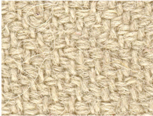
Figure 8. Wool fabric (s2) treated with alkaline protease enzyme.
