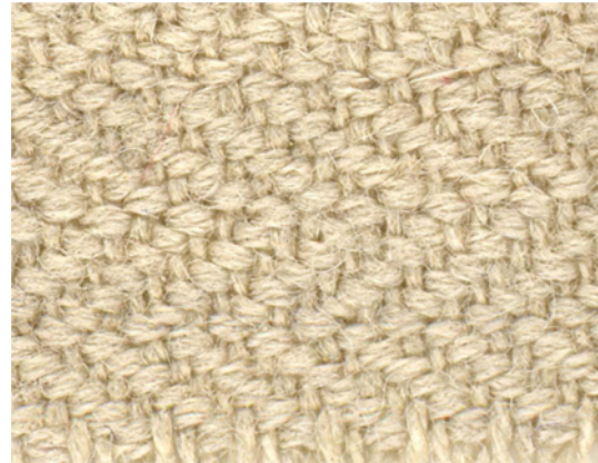
Figure 9. Wool fabric (s1) treated at acid protease and cellulase enzyme.
