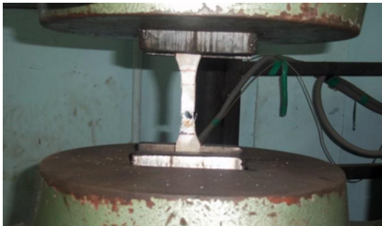
Figure 1. Tensile test specimen after breaking.
