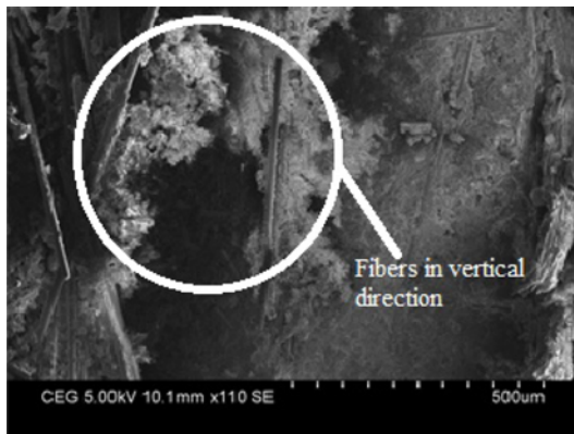
Figure 19. SEM image of sample 3 after tensile test.
