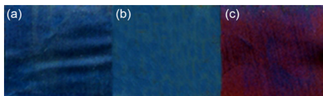
Figure 5. The structural colors in 7 cycles on polyester fabrics with various SiO 2 particle size in (a) 70 nm, (b) 100 nm, and (c) 160 nm.
