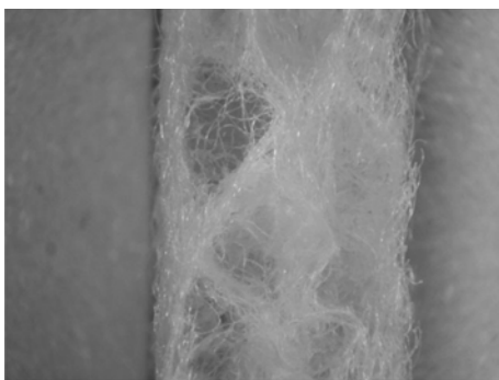
Figure 2. Structure of aerogel treated nonwoven fabrics.
