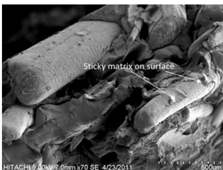
Figure 7. The fracture surface of SPF-HIPS composites with addition 3 % MAH.
