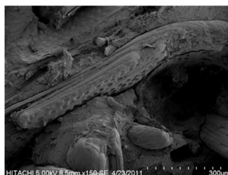
Figure 8. The fracture surface of SPF-HIPS composites with 4 % alkali treated.
