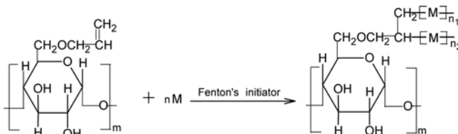
Scheme 2. Formation of the grafted branches through incorporating double bonds into the grafted branches by Fenton's initiator. M denotes the vinyl monomers.
