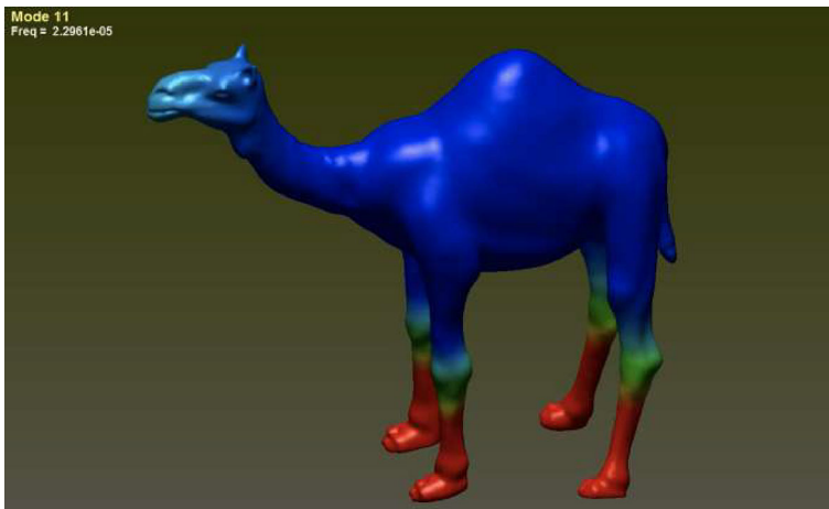
Fig. 52 This is Mode 11. This shows again a 4-legged motion, where the two fore legs are moving back-and-forth, while the two hind legs are moving laterally side-to-center. But the relative motion between the fore and hind legs are out-of-phase in comparison with that of Fig. 51. Once again, these directions of the two types of motion seem to be “orthogonal” to each other. For video animation, please click https://drive.google.com/file/d/1LpaYxuSA46AnyLGU8D4X6jgoaeChD58c/view?usp=sharing
