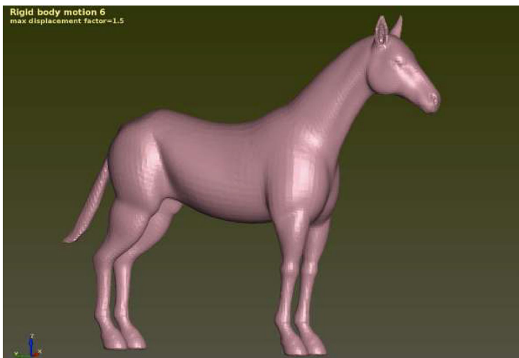
Fig. 11 This is Mode 6 in (5.1) showing a roll rotational rigid body motion. For video animation, please see https://drive.google.com/file/d/1hQ2XH-426HYKtBDRnB6Jfu0U5sF9nMD_/view?usp=share_link
