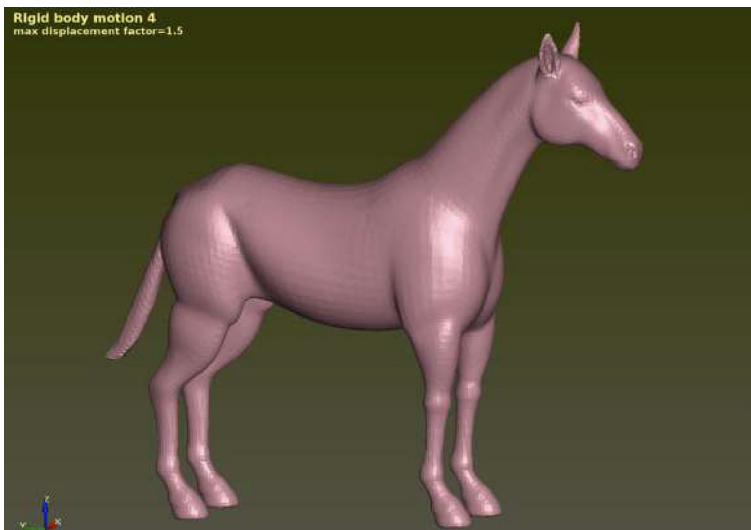
Fig. 9 This is Mode 4 in (5.1) showing a yaw rotational rigid body motion. For video animation, please see https://drive.google.com/file/d/1AbjgtzwFUhsGNsslDslpBpG9wDjEnXL/view?usp=sharing
