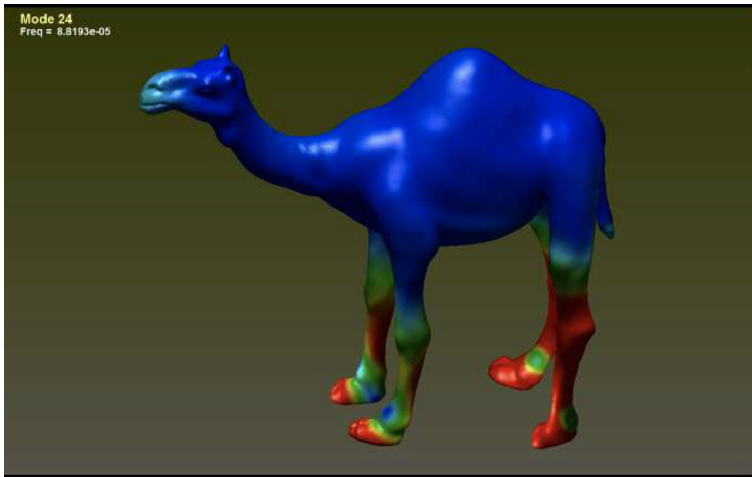
Fig. 65 This is Mode 24. The major motion is the tramping of the hind legs. There is also a minor rotation of the fore feet in the same orientation. For video animation, please see https://drive.google.com/file/d/1QO3Qcv3rkEvTc8M-9RdEiJ7Cf7TWvSw9/view?usp=sharing
