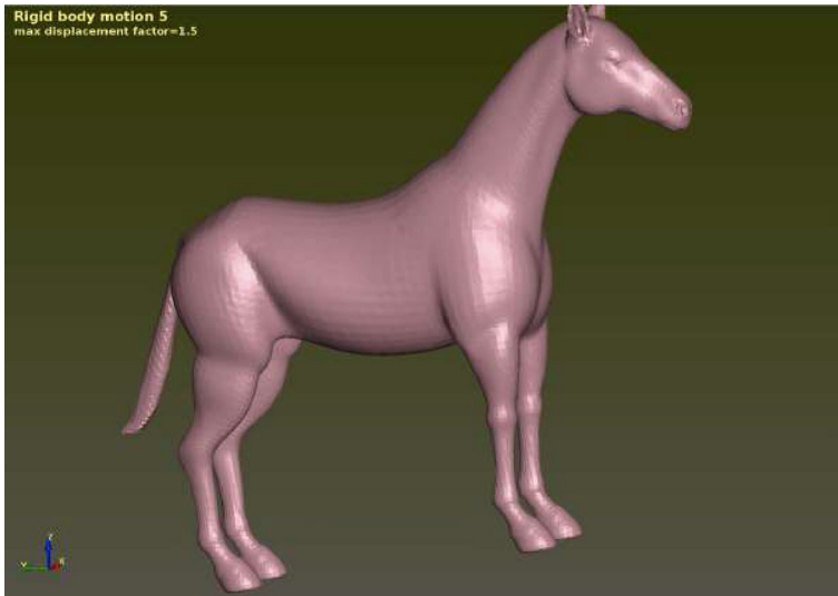
Fig. 10 This is Mode 5 in (5.1) showing a pitch rotational rigid body motion. For video animation, please see https://drive.google.com/file/d/1siy5GzXLfUC1mCpyVizLr-c01jYICivs/view?usp=sharing
