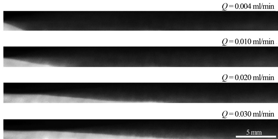
Fig. 3 Concentration field of Rhodamine shown for different values of the volume flow rate. The mixture parameters are the same as in Fig. 2. Figure presents raw images that have not yet been processed
