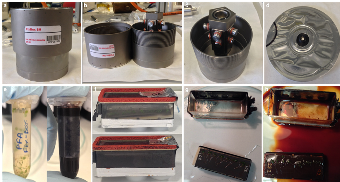
Fig. 5 Science Verification Test (SVT). a Scientific model (SM) of the FixBox. b It is composed of a base and a cover. c Carousel where the five cassettes of each EC are placed, connected through the temperature and hydration ports. d Bag that contains 9 mL of the corresponding fixative solution. e Seedlings fixed in a microfuge tube with and without ferrofluid
