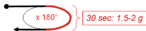
Fig. 3 Aresti diagram of the high bank curve or turn flight maneuver with the Grob G103 Twin II glider plane
