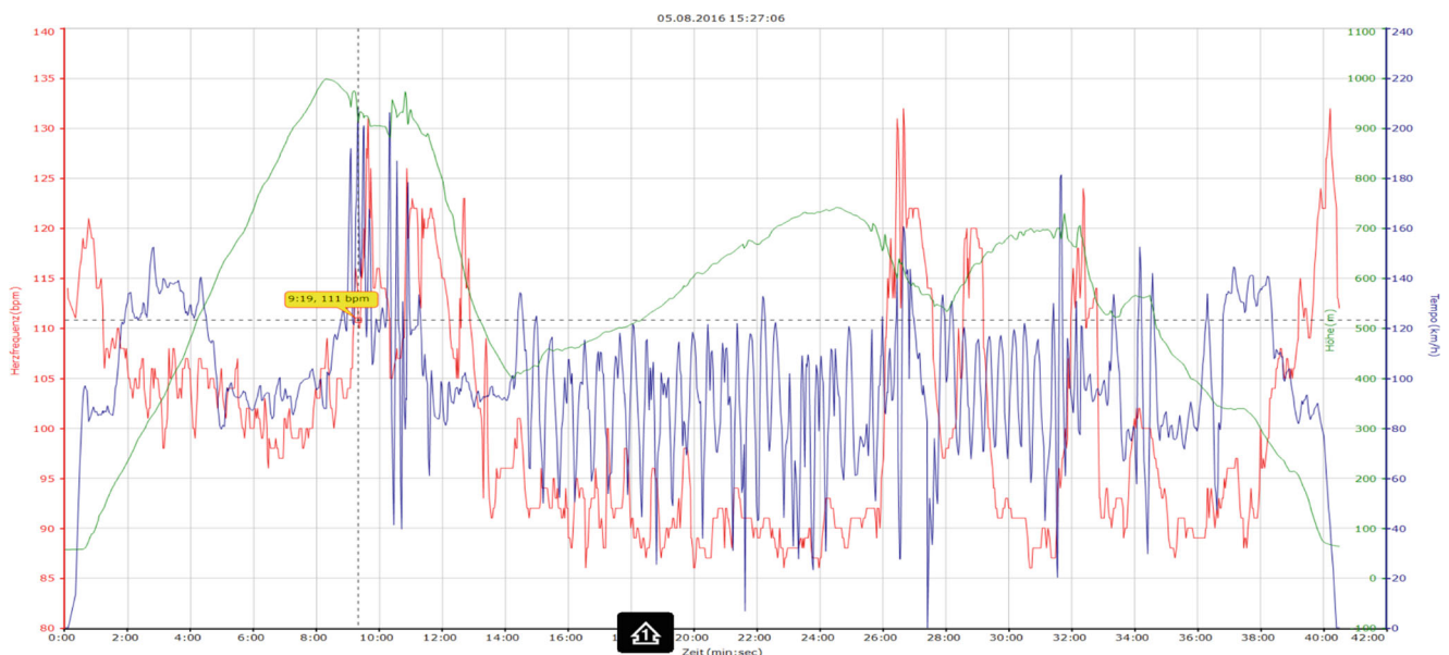
Fig. 8 Print of the Garmin Forerunner 410 Log for a subject. The green curve represents the altitude (full scale: –100 to 1100 m with respect to the ground level), the blue curve the airplane velocity (scale:
