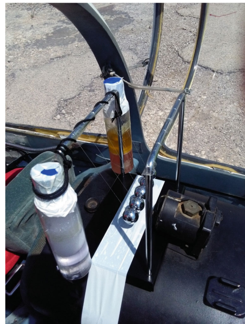
Fig. 4 Newton's cradle pendulum and two small plastic containers with liquids fixed to the pendulum structure. The whole set is attached on top of the glider back seat instrument panel. (Photo: V. Pletser)
