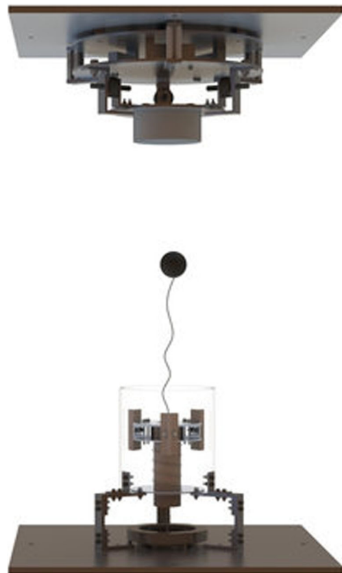
Fig. 7 Docking system using a tether tested in microgravity (Picture: FELDs team)
