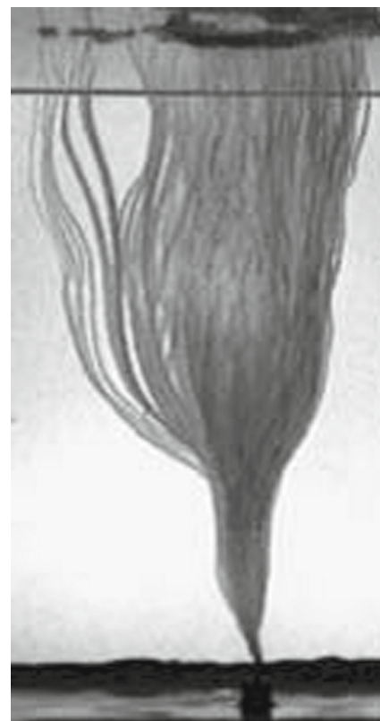
Fig. 10 Image obtained overlapping the frames of each video of rising bubbles (Picture: Bubble Movers team)
