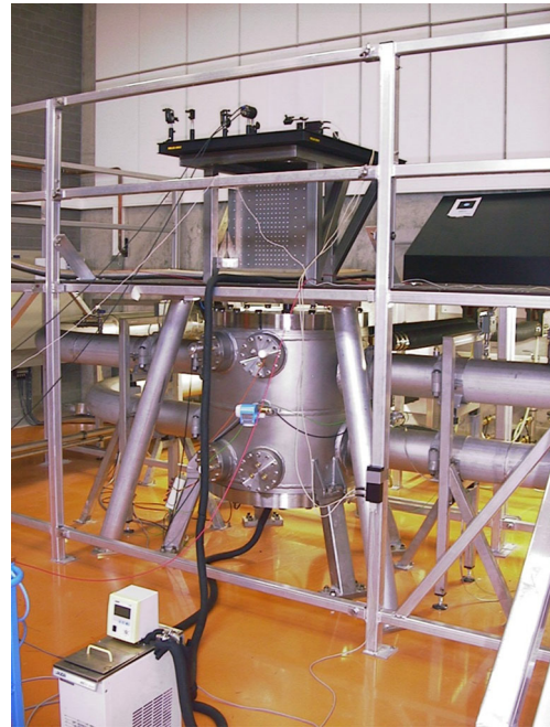
Fig. 12 A picture of a 33 T poly-Bitter magnet of the High Field Magnet Laboratory, Nijmegen. The magnet consists of four electrical coils mounted inside a 1m-diameter, 1m-high cylindrical housing. At maximum field, the electrical current is about 37000 A using a power of 17 MW. The magnet is cooled by cold water ( 12^\circ\text{C} ) at a flow rate of 145 l/s. Access to samples and in situ measurement equipment is possible from above and below the magnet, inside a 32 or 50 mm-diameter vertical bore
