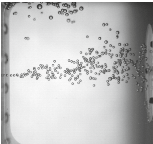
Fig. 1 Snapshot of a typical experiment of slug bubble injection after 2.5 seconds of microgravity
