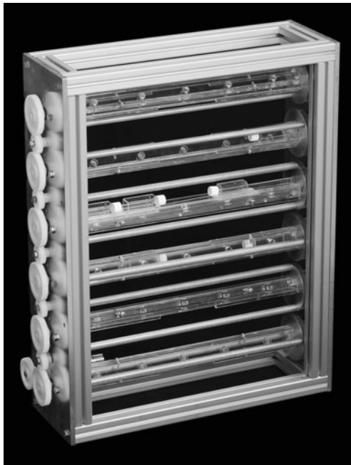
Fig. 4 New clinostat set-up, which can be used as insert for incubators. The clinostat set-up is equipped with 6 parallel rotating axes that can be loaded with 24 slide flasks in total (Design M. Görög, Institute of Aerospace Medicine, DLR, Cologne, Germany)
