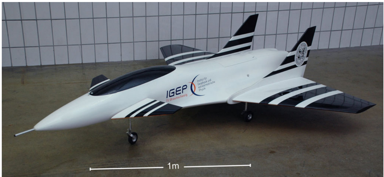
Fig. 4 Our UAV with a maximum take-off weight of 25 kg, a wingspan of 2 m and a length of 2.5 m, designed for a flight speed of 100 \text{ m s}^{-1} and an acceleration of 5 g_0
