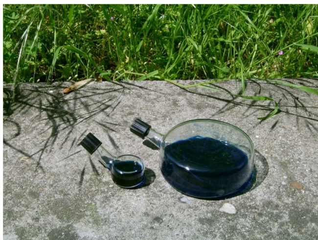
Fig. 2 (left) Reaction vessels employed for sunlight-promoted TBADT-photocatalyzed C–H alkylations. Adapted from (Protti et al. 2009) with permission from The Royal Society of Chemistry.
