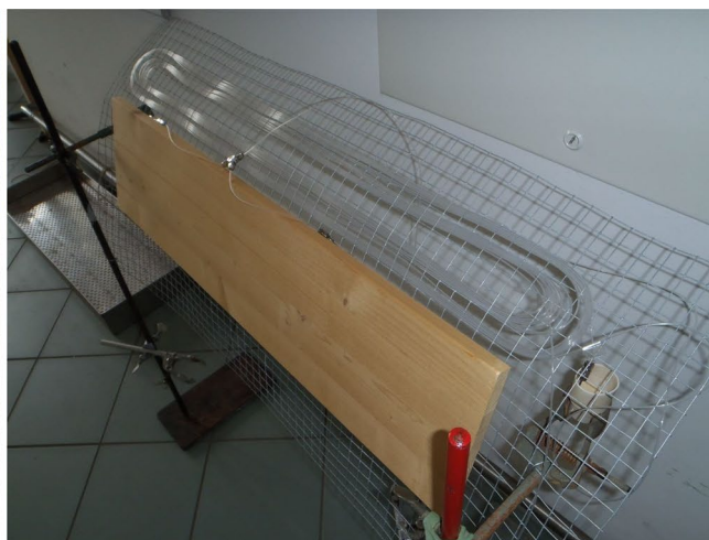
(right) The “sunflow” apparatus adopted for the benzophenone-promoted functionalization of benzoxazoles. Reproduced with permission from (Nauth et al. 2017)
