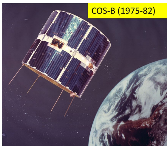
Fig. 2 COS-B (1975–82): imaging telescope ( E > 70 MeV) with a central digital wire spark chamber (about 24 \times 24 cm 2 in size, with 16 gaps, interspersed with thin Tungsten layers for pair conversion).
