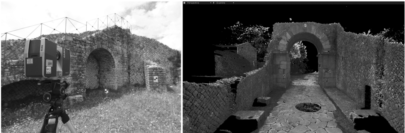
Fig. 1 The laser scanning survey of the archeological site of Sepinum (Italy) done during the Summer School organized by the Laboratorio di Fotogrammetria of the Università Iuav di Venezia in July 2014
