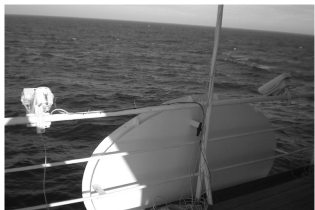
Fig. 1 Example of a stereo system (WASS) installation to measure sea surface waves. The two cameras composing the stereo rig are down-looking and about 2.5 m apart
