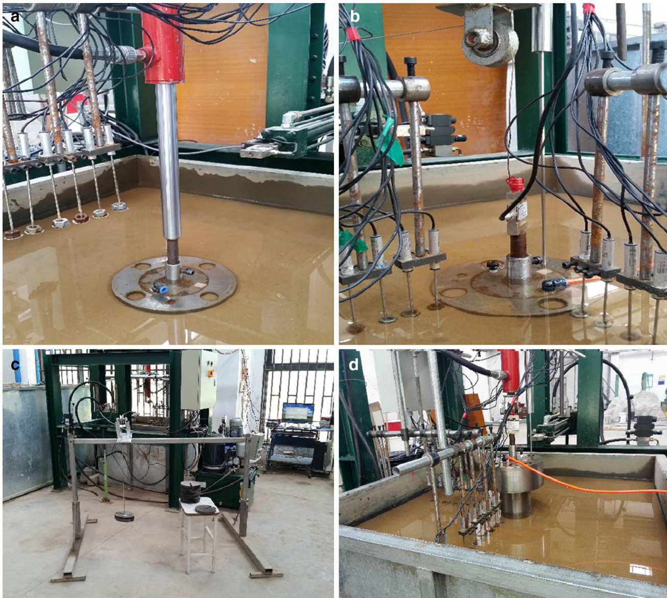
Fig. 3 Procedure of the test. a Suction caisson installation, b transducers, c stepped loading, d suction caisson pullout in progress
