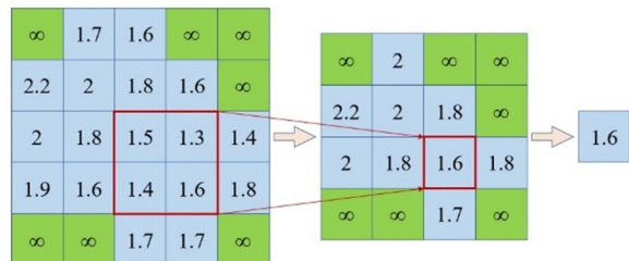
Fig. 4. The worst-best subsampling method ( \infty means the configuration is unreachable for the manipulator).
