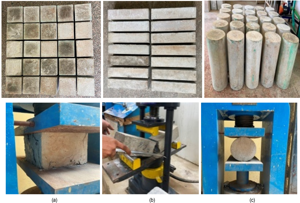
Fig. 2. Testing of various samples: (a) compressive strength cubes; (b) flexural strength beam; (c) splitting tensile strength cylinder.
