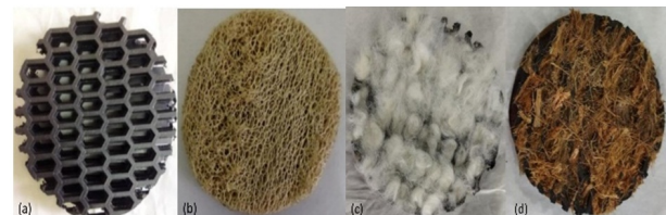
Fig. 3. The combination of BC-MPP backed with (a) honeycomb structure; (b) loofah; (c) honeycomb structure filled kapok; (d) honeycomb structure filled coconut coir.
