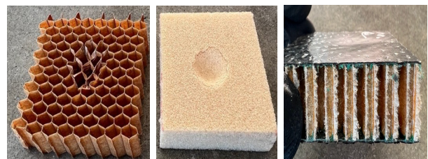
Fig. 6. Damage after indentation.
