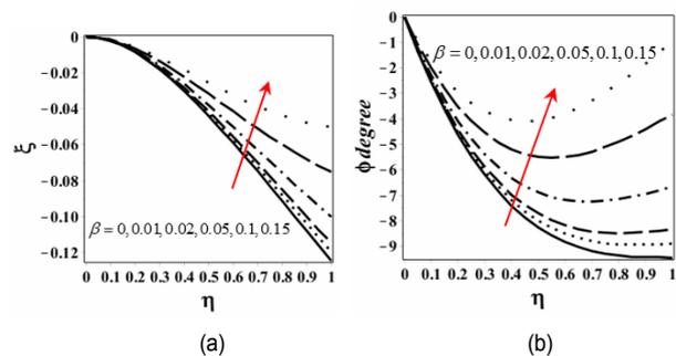
Fig. 6. (a) Variation of the vertical deflection  $\xi$  of the cantilever nano-beam vs. the dimensionless longitudinal distance  $\eta$ ; (b) variation of the bending angle  $\varphi$  vs. the longitudinal distance  $\eta$ , based on the nonlocal elasticity theory considering the nonlinear curvature for  $\alpha = 1$  and  $k_1 = k_2 = k_s = 0$  and different values of the nonlocal parameter  $\beta = 0, 0.01, 0.02, 0.05, 0.1$  and  $0.15$ .
