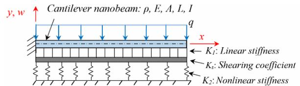
Fig. 1. A thin cantilever nano-beam on a nonlinear Winkler-Pasternak elastic foundation and under uniformly distributed lateral load.
