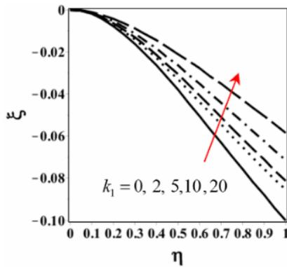
Fig. 8. Variation of the vertical deflection  $\xi$  of the nano-beam versus the dimensionless longitudinal distance  $\eta$  based on the nonlocal elasticity theory considering the linear curvature for  $\alpha = 1$ ,  $\beta = 0.05$ ,  $k_2 = k_s = 0$  and different values of the linear stiffness coefficient of the foundation  $k_1 = 0, 2, 5, 10$  and  $20$ .
