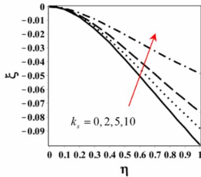
Fig. 11. Variation of the vertical deflection  $\xi$  of the cantilever nano-beam versus the dimensionless longitudinal distance  $\eta$  based on the nonlocal elasticity theory considering the nonlinear curvature for  $\alpha = 1$ ,  $\beta = 0.05$ ,  $k_1 = k_2 = 0$  and different values of the shear stiffness coefficient of the foundation  $k_s = 0, 2, 5$  and  $10$ .
