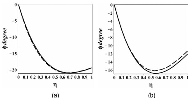
Fig. 5. Variation of the bending angle  $\varphi$  of the cantilever nano-beam versus the dimensionless longitudinal distance  $\eta$  based on nonlocal elasticity theory with  $\alpha = 3$  and  $k_1 = k_2 = k_s = 0$ : (a)  $\beta = 0.05$ ; (b)  $\beta = 0.1$ , ----- linear curvature (dashed line), — nonlinear curvature (solid line).
