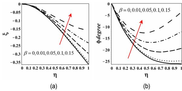
Fig. 7. (a) Variation of the vertical deflection of the nano-beam versus the dimensionless longitudinal distance; (b) variation of the bending angle versus the longitudinal distance based on the nonlocal elasticity theory considering the nonlinear curvature for  $\alpha = 3$  and  $k_1 = k_2 = k_s = 0$  and different values of the nonlocal parameter  $\beta = 0, 0.01, 0.05, 0.1, 0.15$ .
