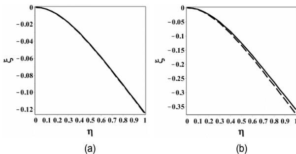
Fig. 4. Variation of the vertical deflection  $\xi$  of the classical cantilever Euler-Bernoulli versus the dimensionless longitudinal distance  $\eta$  using linear and nonlinear curvature for  $\beta = 0$  and  $k_1 = k_2 = k_s = 0$ : (a)  $\alpha = 1$ ; (b)  $\alpha = 3$ , ----- linear curvature (dashed line), — nonlinear curvature (solid line).
