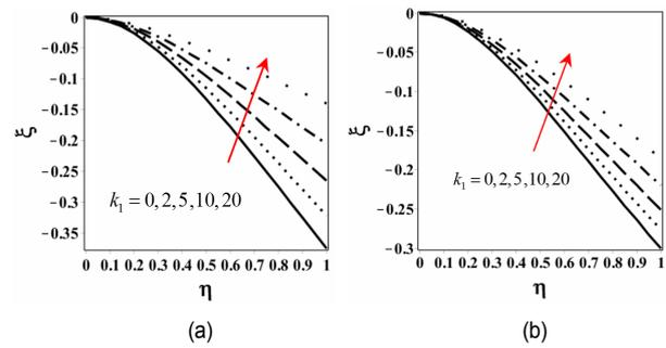
Fig. 9. Variation of the vertical deflection  $\xi$  of the cantilever nano-beam versus the dimensionless longitudinal distance  $\eta$  based on classical and nonlocal elasticity theories considering the linear curvature for  $\alpha = 3$ ,  $k_2 = k_s = 0$  and different values of the linear stiffness coefficient of the foundation  $k_1 = 0, 2, 5, 10, 20$ : (a)  $\beta = 0$ ; (b)  $\beta = 0.05$ .
