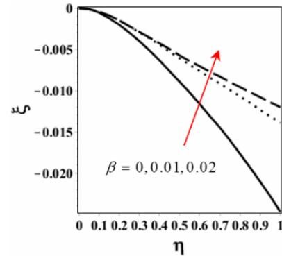
Fig. 13. Variation of the vertical deflection  $\xi$  of the cantilever nano-beam in terms of the dimensionless longitudinal distance  $\eta$  based on the nonlocal elasticity theory considering the linear curvature for  $\alpha = 1$ ,  $k_1 = 100$ ,  $k_2 = 50$ ,  $k_s = 20$  and different values of nonlocal parameter  $\beta = 0, 0.01$  and  $0.02$ .
