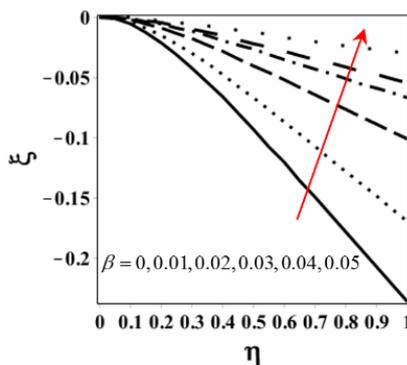
Fig. 12. Variation of the vertical deflection  $\xi$  of the cantilever nano-beam versus the dimensionless longitudinal distance  $\eta$  based on the nonlocal elasticity theory considering the nonlinear curvature at  $\alpha = 1$ ,  $k_1 = 100$ ,  $k_2 = 50$ ,  $k_s = 20$  and different values of the nonlocal parameter  $\beta = 0, 0.01, 0.02, 0.03, 0.04$  and  $0.05$ .
