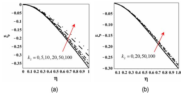
Fig. 10. Variation of the vertical deflection  $\xi$  of the cantilever nano-beam versus dimensionless longitudinal distance  $\eta$  based on the classical and nonlocal elasticity theory considering the linear curvature for  $\alpha = 3$ ,  $k_1 = k_s = 0$  and different values of the nonlinear stiffness coefficient of the foundation  $k_2 = 0, 5, 10, 20, 50, 100$ : (a)  $\beta = 0$ ; (b)  $\beta = 0.05$ .
