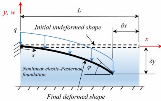
Fig. 2. The effect of length change of a thin nonlocal cantilever nano-beam considering the bending large deflection under uniformly distributed lateral load (in which is always perpendicular to the initial longitudinal direction of the beam) and on a nonlinear Winkler-Pasternak elastic foundation.
