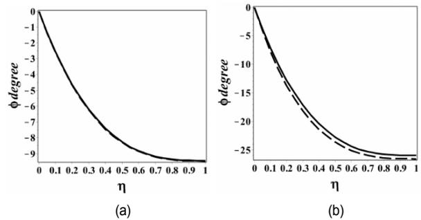
Fig. 3. Variation of the bending angle  $\phi$  of the classical cantilever Euler-Bernoulli beam versus the dimensionless longitudinal distance  $\eta$  without foundation ( $k_1 = k_2 = k_s = 0$ ): (a)  $\alpha = 1$ ; (b)  $\alpha = 3$ , ---- linear curvature (dashed line), — nonlinear curvature (solid line).
