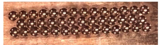
(e) Indentation test at 1 indent diameter spacing for 9.525-mm-thick copper (3 rows)
