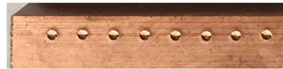
Fig. 7. This figure shows e equal to 2 indentation diameters for the 9.525-mm-thick copper.
